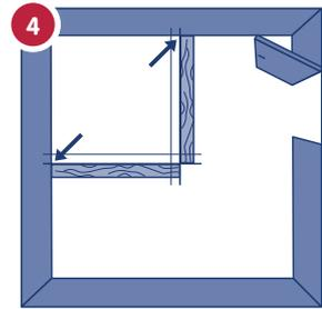
4 Mark the new starting point and transfer these marks to the corresponding skirting boards or walls. Position straight edges on these marks in both directions.
