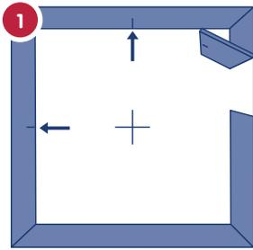
1 Determine the centre point of the room and mark it. Transfer these marks to the corresponding skirting boards or walls.
