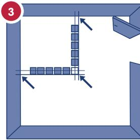
3 If cut tiles are too small, move the centre tile so that the middle of the tile coincides with the centre mark on the floor. Repositioning the tiles will now ensure correct cuts.
