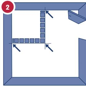
2 Starting at the centre mark, place a row of loose tiles along these lines. Cut tiles should be at least half a tile wide. If this is the case, position straight edges as per step 4. Remember to leave room for tile spacers, tile panel movement joints and perimeter joints.
