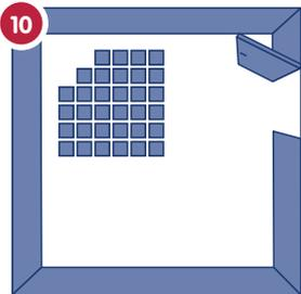
10 Tile out from the centre mark to the edges, keeping lines straight and tile spacing even. Leave cut tiles until last.
